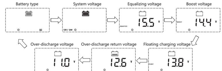
After entering into the setting interface, tap the Set key to switch the menu for setting, and tap the Up or Down key to increase or decrease the parameter value in the menu. Then tap the Return key to exit (without saving parameter setting), or press and hold the Set key to save setting and exit.
