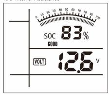
SOC: State of Charge VOLT: Battery Voltage
