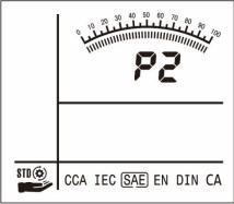
D. Hold the or to select the battery EDC/CCA values(specified on the battery rating label or Refer to the EDC/CCA Parameters Table)
