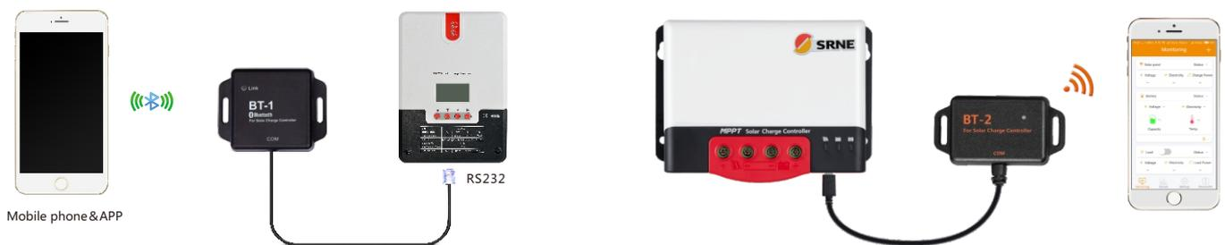
**Note:** use a standard network cable (parallel cable) for connection.
