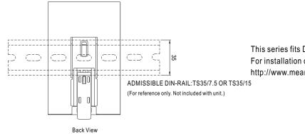
This series fits DIN-RAIL TS35/7.5 or TS35/15. For installation details, please refer to the USER MANUAL on http://www.meanwell.com/search/NDR-480/NDR\_manual.pdf
