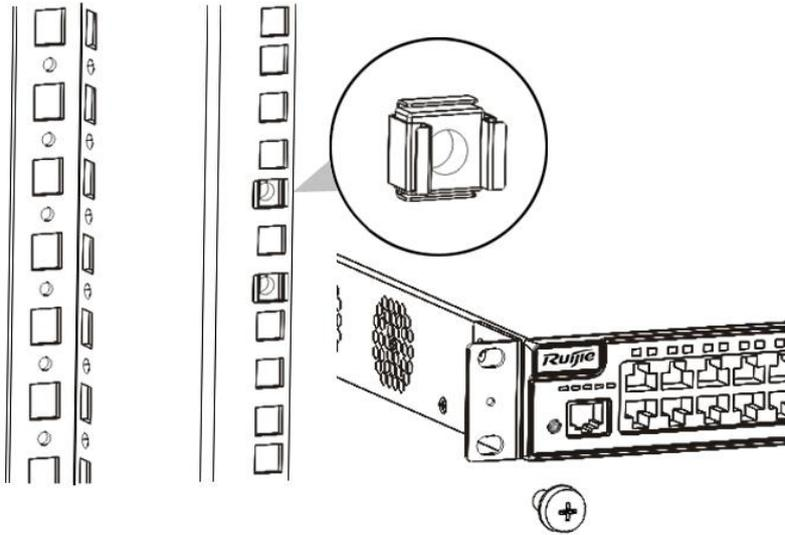
Figure 3-3 Attaching the Brackets to the Rack
