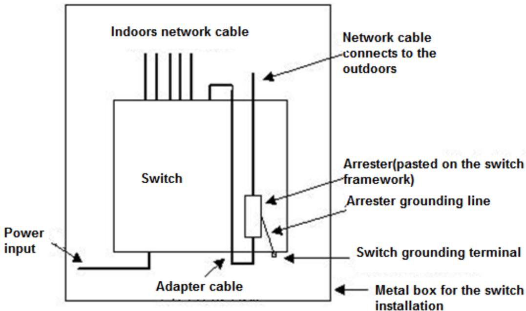
⚠ The Ethernet port arrester applies to only the 10M/100M electrical Ethernet ports with the RJ45 connector.
