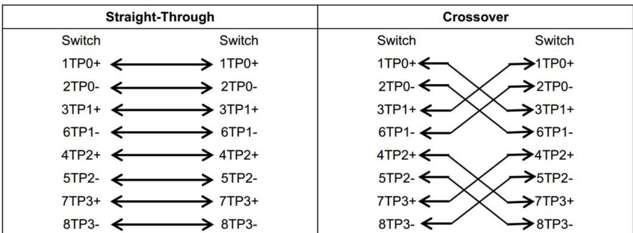
In addition to the preceding cables, the 100BASE-TX/10BASE-T can also use 100-ohm Category-3, Category-4, and Category-5 cables for 10 Mbps, and 100-ohm Category-5 cables for 100 Mbps, both of which can be up to 100 m.
