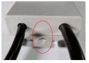
**Ground** Make sure that the grounding end of the product is well connected to the earth through the grounding wire (self-provided).
