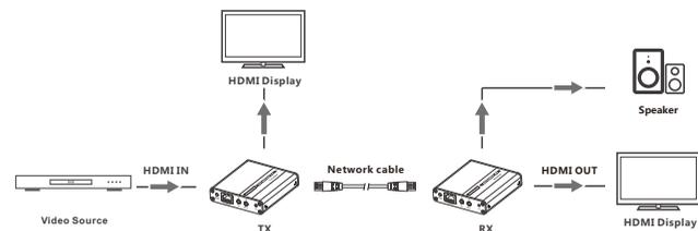
**Note:** When using the 3.5mm stereo audio jack, please switch the audio output format of the signal source to PCM format.
