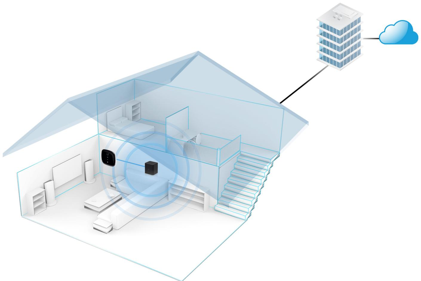
*The UFiber Active Ethernet delivers active fiber from the service provider to the customer's residence, where it is powered by the airCube™ AC, model ACB-AC.*
