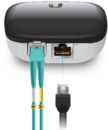
*Connect an Ethernet cable from a device
