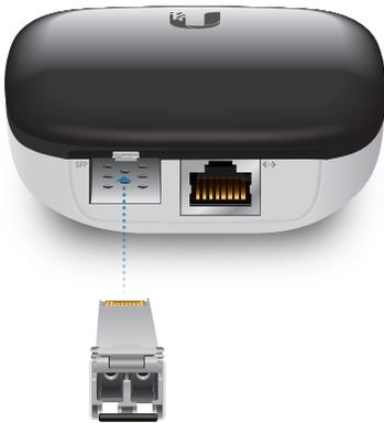
*Insert a compatible active fiber SFP module.
