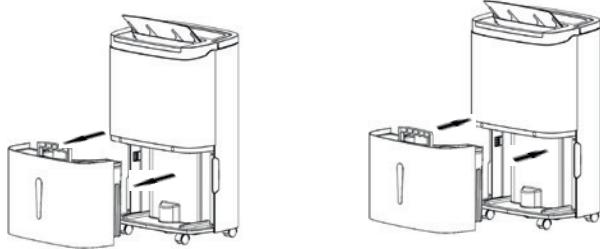
the dehumidifier, please confirm whether the floater rotates flexibly or not, then put it in position using both hands.
