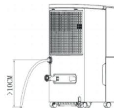
Attention: the level height of externally connected water pipe shall not be higher than the water outlet, and the water pipe at rear-end shall transit smoothly, otherwise the leakage risk exists since drainage is not smooth.
