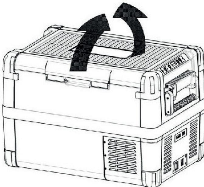
The lid can be removed, or can be opened from both sides, 2 ways for opening – left or right.
