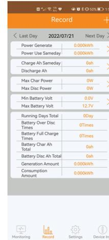
The lowest and highest battery voltage of the day can be displayed in real time;
