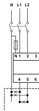
**Fig. 7** Two-phase (3-wire).
