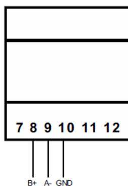
**Fig. 11** RS485 port
